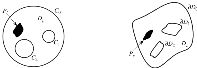
FIGURE 1. The idea of the algorithm: a conformal map z(\zeta) transplants a circular pre-image domain D_\zeta to the physical fluid region D_z containing a vortex patch P_z . The pre-image of P_z in D_\zeta is P_\zeta .
